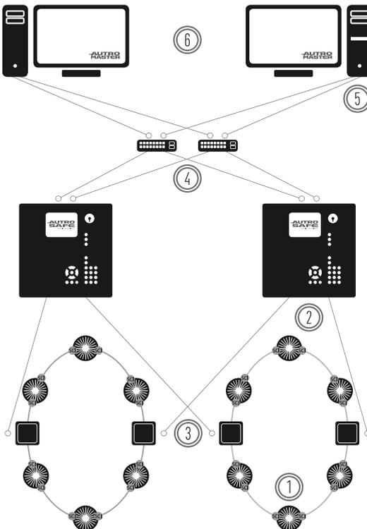
Should one panel fail due to a fire incident, the other will maintain control.
