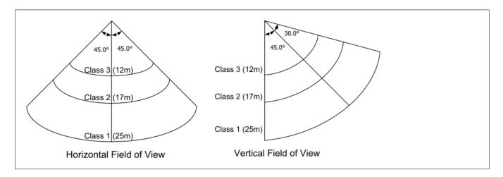
To comply with the directional dependence requirements for EN 54-10:2002 an angle of  $\pm 30^{\circ}$  from 0° (0° = Orientation of detector in same axes as flame source) should not be exceeded, based on lab testing at a distance of approximately 5.0 ft (1.5 m).
